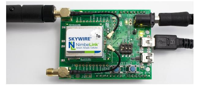
The J14 interface will connect to the modem's USB to serial UART interface IC to access the modem's serial UART interface. The D3 LED will illuminate when USB is connected.
