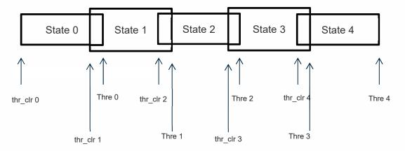
When temperature exceeds the "current state" "threshold", the thermal mitigation algorithm searches the next state that this temperature is lower than its "threshold". After it finds it, the "current state" is updated to that "state" and then it checks whether "action" is "mitigate", if yes, then it activates the mitigation according to the "action info" of the "current state".
