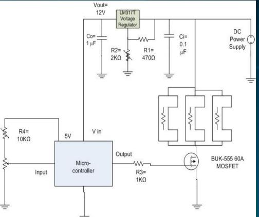
Drawing-1. Electromagnetic Brake System Circuit Diagram
