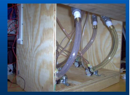
The pump will draw liquid from the bottle and distribute the liquid into the user's glass
