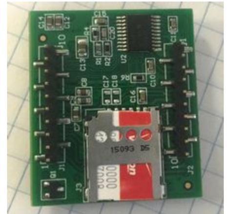
3. Line up your Skywire's™ cellular U.FL connector(s) on the side of the board closest to the antenna connector. Then carefully seat your Skywire™ into the board's Skywire™ socket (U1). Take care to ensure that the pins are correctly aligned. Failure to properly align the pins may damage your Skywire™.
