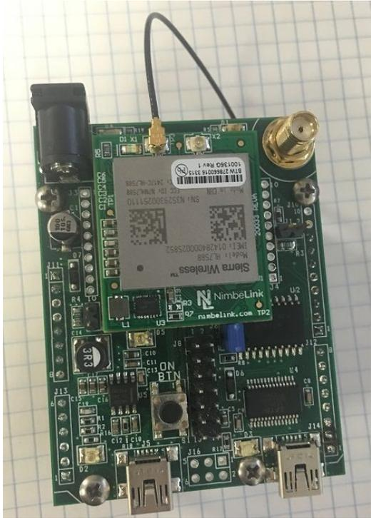
A properly mounted Skywire™ Modem with U.FL cable attached to top U.FL connector X1
