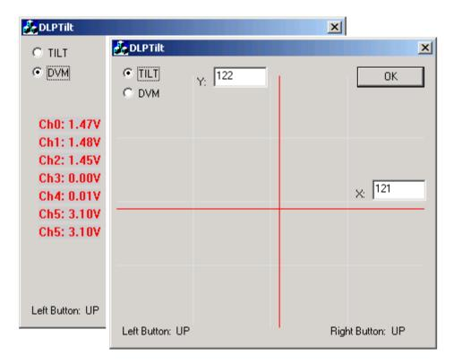
This program is designed to both demonstrate the tilt feature of the accelerometer and present the acquired voltages from each of the seven analog inputs.
