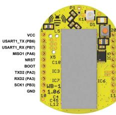
ON/OFF (PA0) DAC/AIN3 (PA10) **GPIO3 (PA15)** CS1 (PB2) SDA1/AN1(PB14) SCL/AIN0 (PB13) VREF P ON/SLEEP (PC13) CTS1/AIN7 (PA11) MOSI1 (PB5)
