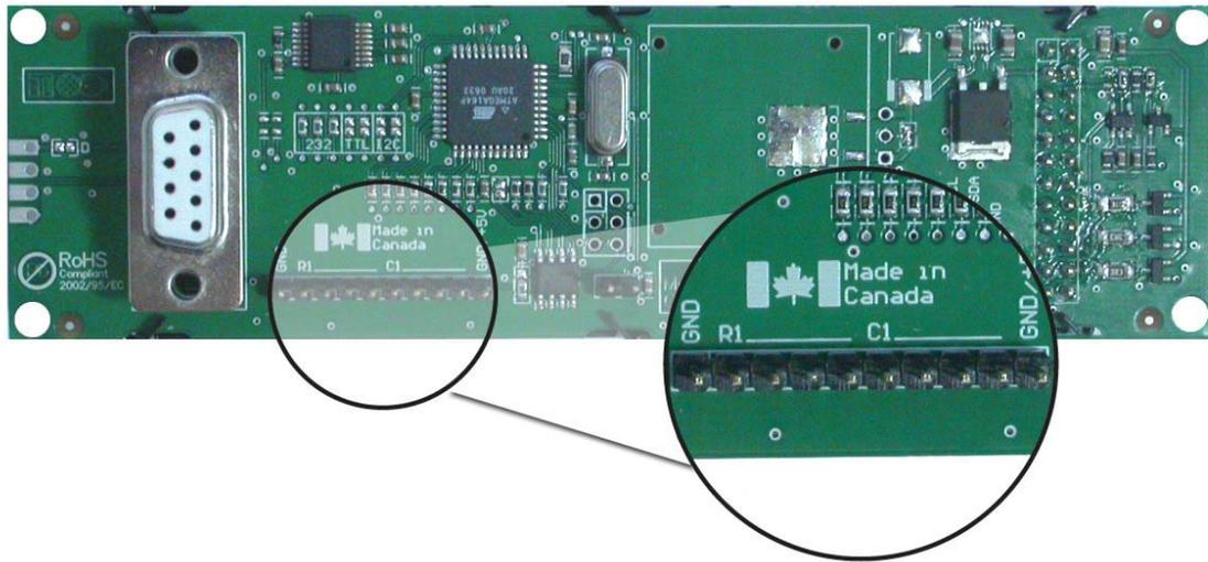
Figure 16: Keypad Interface Connector
