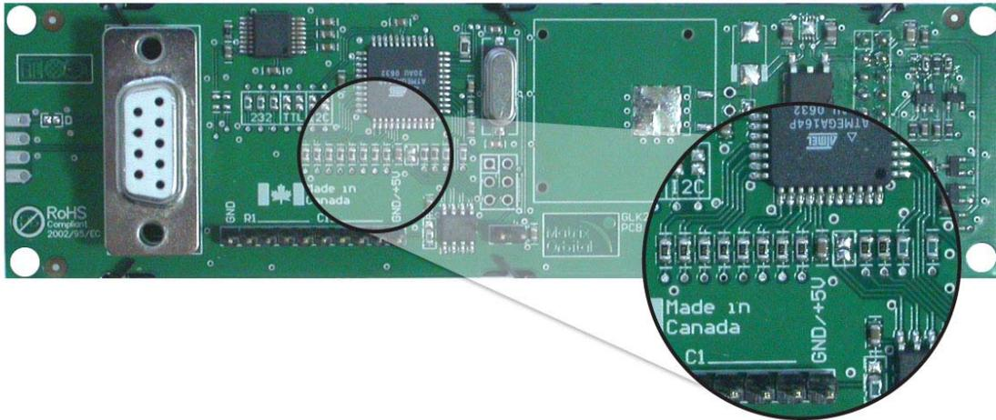
Figure 19: Filesystem Lock Jumper
