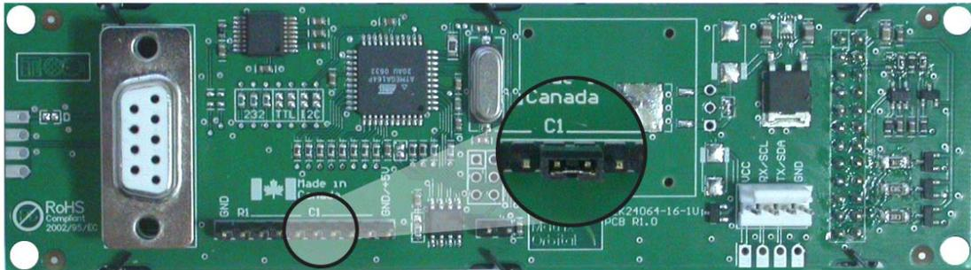
Figure 18: Manual Override Jumper
